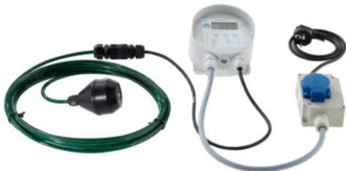
With this LINN- monitoring system you have the opportunity, to measure and control dissolved oxygen in a single pond. The oxygen level is measured by an oxygen probe steadily. If the adjusted alarm level is exceeded or undershot, an additional plugged system can set off an alarm and can goose or power off plugged devices. The adjustment of the alarm levels is easy with the accompanying control. Please note the following points.
